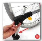
The anti-tip wheels prevent the wheelchair from tipping backwards. The anti-tip castors must have a distance of approx. 3-5 cm from the floor (Fig. 35).
