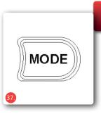
The user can activate the adjustment functions with the Mode button. The lamps for the relevant LED for an adjustment option (left footrest, right footrest, seat, backrest) show which adjustment function is active at that time.
